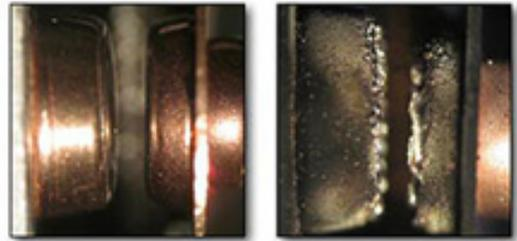
In addition, pitting creates opposing hills and valleys on the contact surfaces in the area where melted metal is transferred by the electron flow. Couple these uneven contact surfaces with a small amount of over-travel built into the closing contacts of the relay, and you soon have metal-on-metal ledges lodged against valleys. Combine that with heat via contact resistance from applied current, and the contacts will eventually stick.
